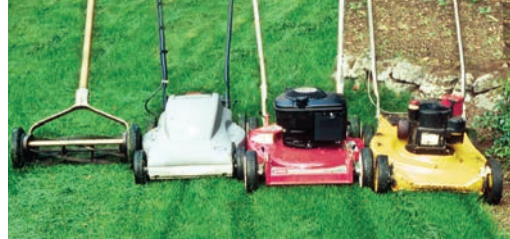
Electric and gas "mulching" mowers (center) chop clippings and blow them down to soil to decompose.
